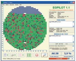
Electroglas semiconductor Prober control software with wafer mapping and zoom capability.
